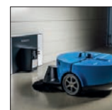
Station de recharge
