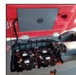
Compartment des batteries
